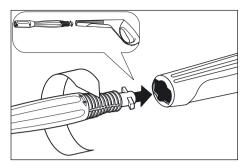
**Step 2**Insert the variopower nozzle into the trigger gun. Press in against the spring tension and twist into the locked position.
