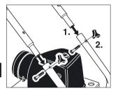
**Step 1**Attach the handle to the frame of the pressure washer. Align holes, insert bolts, and
